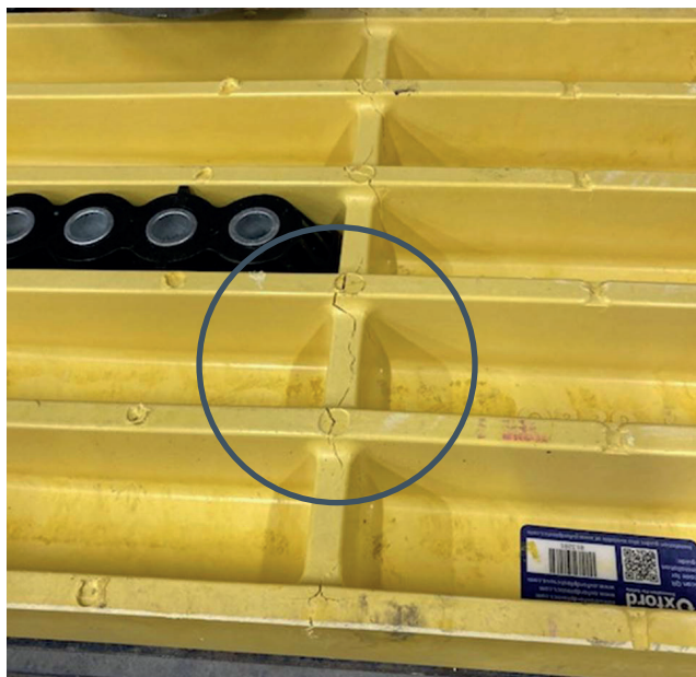
Crack along rib
